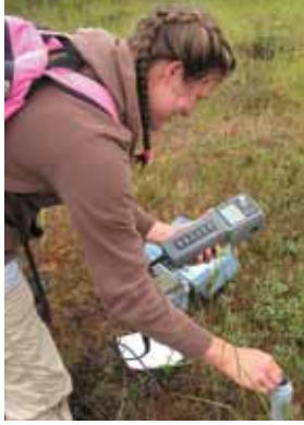
Kaysha measures dissolved oxygen in a well pipe. These wells are the source of sub-surface water samples and make up the sampling network, along with surface water sites.
